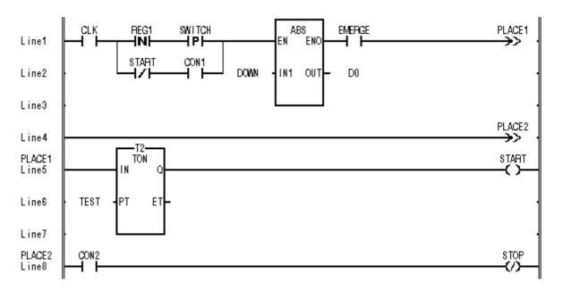
☐ The function and function block can be located everywhere at LD. Connecting power flow line to function and function blocks Input/Output and contact to power flow line can continue the logic operation.
