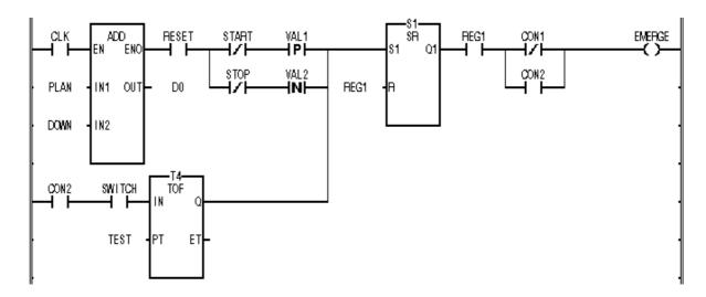
$\square$  The power flow line, which can be connected to one function and one function block, is only one.
