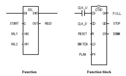
A BOOL type input and output shall be located at each function or function block in order to allow the power flow into the function or function block. EN and ENO is BOOL type Input/Ouput at the function and first input and output is BOOL type at the function block.
