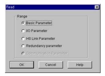
Basic Parameter : Read only a basic parameter from PLC.
