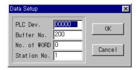
3. Buffer No. is the system buffer number in the PMU main machine
