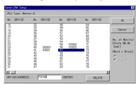
2. After the selection of PLC type, the Serial Link Setup screen below appears.
