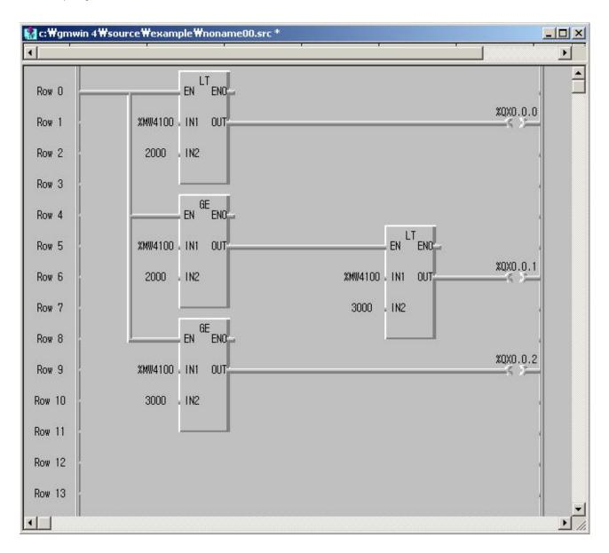
(2) Program which controls speed of inverter by analog output voltage of 5 steps
