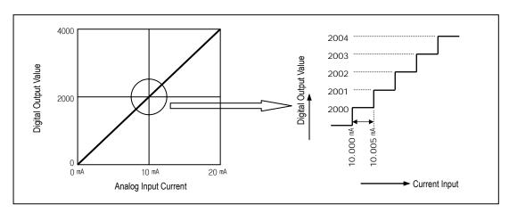
A/D Conversion Characteristics (Current Input  $0 \sim 20$  mA)
