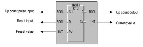
• If the counting value (CV) increments and reaches the setting value (PV), the output contact (Q) turns on. When the reset signal is turn on, the counting value is set to 0' and the output contact (Q) turns off.
