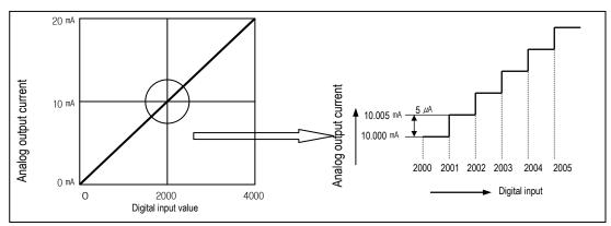
D/A conversion characteristics (Current output)
