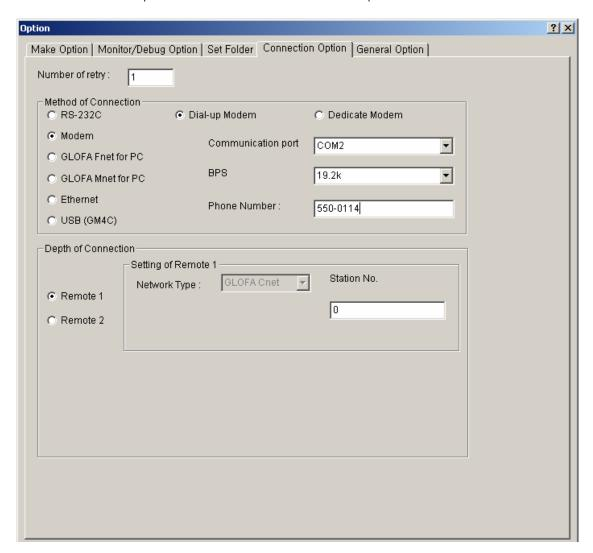
Select Dial-up Modem or Dedicated Modem in Method of Connection, and enter BPS and phone number (Dial-up Modem).
