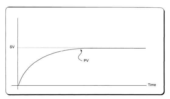
Fig. 7.4 The system response when a long integration time given
