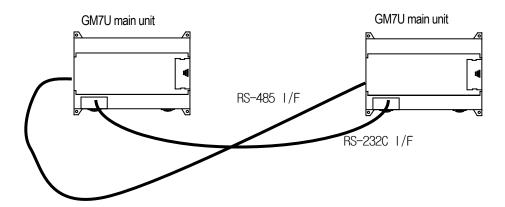
The wiring diagram using RS-232C I/F is as follow.
