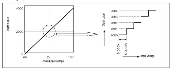
A/D conversion characteristics (voltage input)
