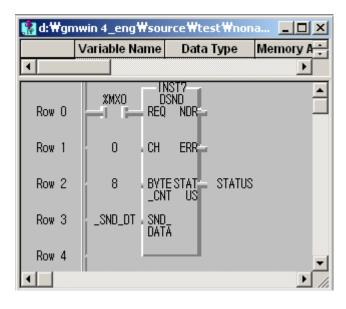
• When the execution condition %MX000 is on, the saved data in \_SND\_DT is sent by 8 bytes via communication channel o.
