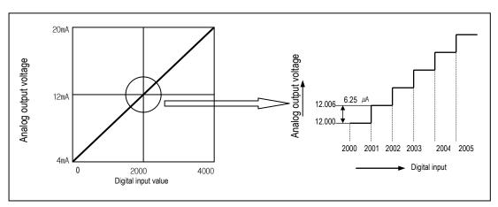
D/A conversion characteristics (Current output)
