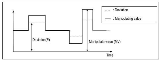
Fig 7.1 MV by P operation
