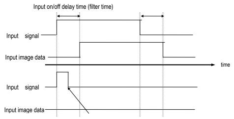
Narrower width pulse than input correction no. is not considered as input signal
