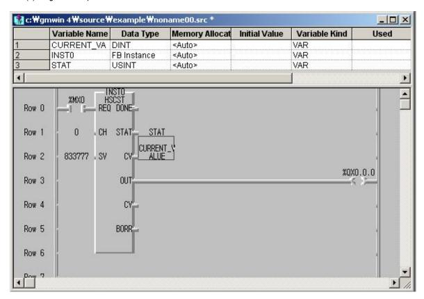
When the input condition %MX000 turns On, the CH 0 is enabled following the set mode.
