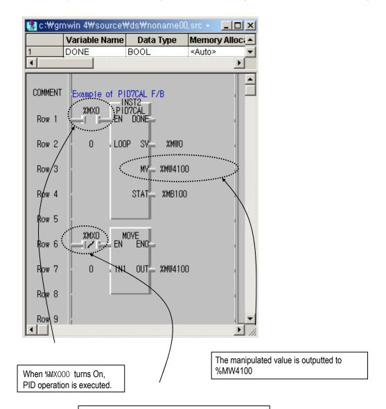
When %MX000 turns Off, 0 is outputted at %MW4100 (Ch0 of DA conversion module)
