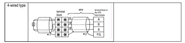
Method of Connection between Pt and RTD Input Module
