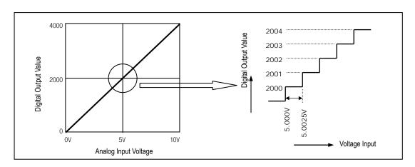
A/D Conversion Characteristics (Voltage Input)
