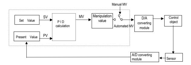
The characteristics of the PID function of GM7U is as following;
