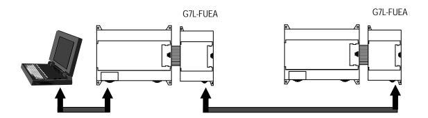
• Remote connection by Fnet interface is available by setting connection options in GMWIN.
