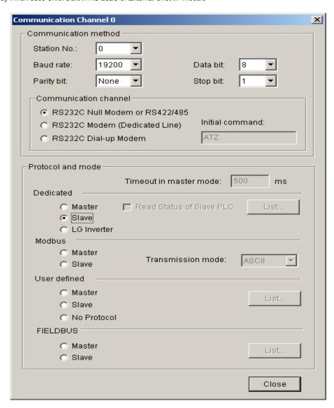
b) When uses Ch.1: Built-in RS-485
