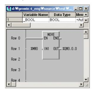
The program of the slave is to output the data at M area to the output contact coil.
