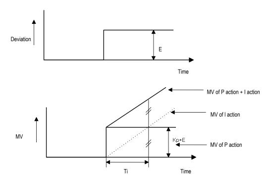
Fig. 7.3 The integral action with constant deviation
