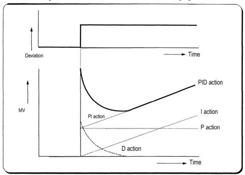
Fig. 7.7 PID action with a constant deviation
