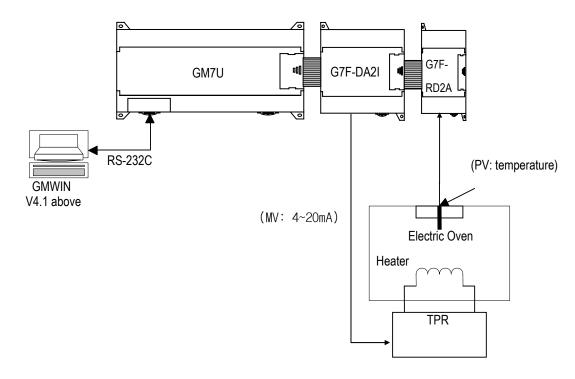
(2) In case of using PID function only
