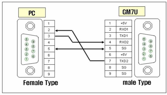
TXD1, RXD1 are for loader communication and TXD2, RXD2 are for Cnet I/F. To use channel 1, connect 485+ and 485- of RS-485 terminal.
