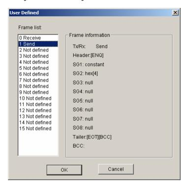
(7) Set up a program like the following figure and download it to the slave station GM7U. For details on program setting and downloading, refer to the GMWIN manual.
