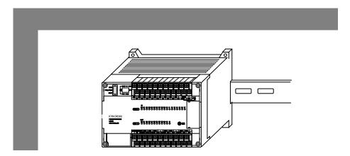
(3) Do not mount the base board together with a large-sized electromagnetic contact or no-fuse breaker, which produces vibration, on the same panel. Mount them on different panels, or keep the unit or module away from such a vibration source
