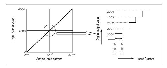
Current input 0mA becomes output 0, 10mA does 2000 and 20mA does 4000. therefore input 5  $\mu$ A equals to digital amount 1, but value less tan 5  $\mu$ A can't be converted. So abandon it.
