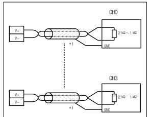
\*1: Be sure to use two-core twisted shield wire.
