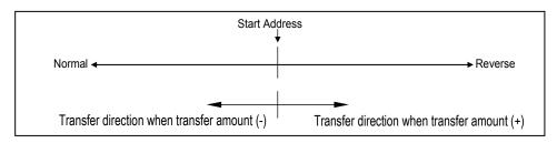
Example) When start address is 5000 and goal address is -7000, this will be reverse direction and positioning will be at the point of 2000
